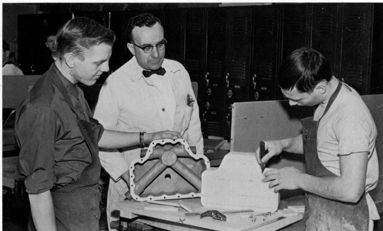
Jerry Houke puts the finishing touches on a pattern for an aircraft engine part while Mr. Robert Larson and Doug Johnson examine his work.
